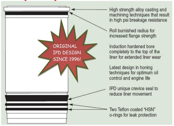
The ORIGINAL IPD CS Cylinder Liner (Crevice Seal) Style Cylinder Liner fro Caterpillar 3406 & C15 engines! Continued...
